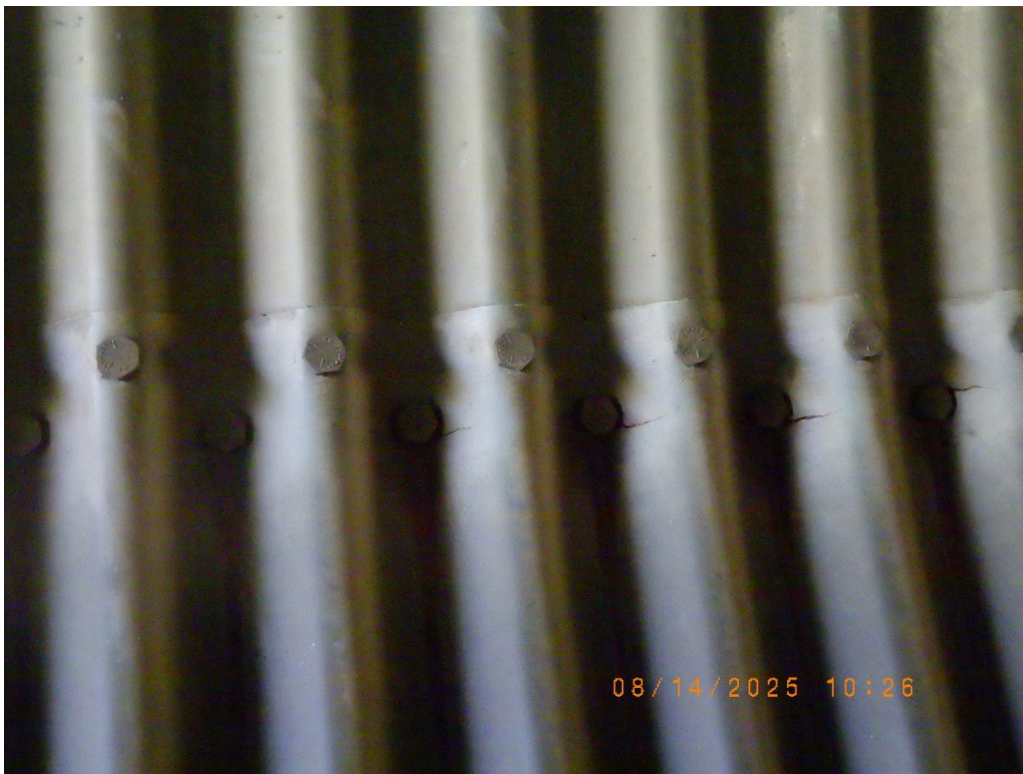
Photo 10: Cracking at bolts inside barrel.
